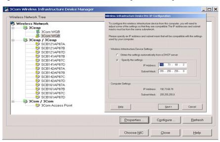
Figure 15 Wireless Infrastructure Device Manager Pre-IP Configuration
